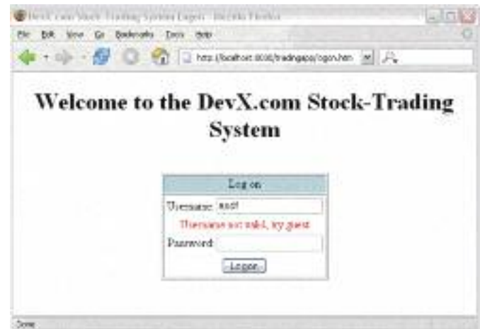
Figure 4. Validating: When the logon page does not validate correctly, the user is returned to the form page where the validation errors are displayed.
